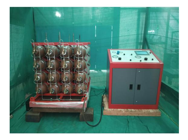
Helium Decanting and Boosting System (Model no. – P1253-PressurePAC) Document Prepared and Published By Paskals Fluid System Pvt. Ltd E-148, Sector-63, NOIDA, UP-201301 Office: Phone: +91-1206524888 and Fax: +91-120-4500888
