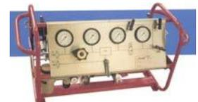
**Gas TestPAC** units have been designed for operators of helicopters and/ or small aircraft where a portable self-powered Booster is needed for ground support. The Pop Floats are inflated from a 3,000 psi (or newer 5,500 psi) bottle housed in the nose of the cockpit. Powered and fed from a standard Nitrogen gas cylinder the **TestPAC** will charge the in-flight bottle. Sometimes Helium is used in preference to Nitrogen because of its faster inflation characteristics.
